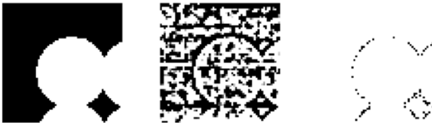
Figure 8.4. Edge detection in incomplete spectral data by zero-crossing. Left : Original image. Centre : Image recovered from incomplete data zero-crossing. Right : Zero-crossing combined with compressive sensing (8.8), with Gaussian concentration factor \Lambda^1 and threshold \zeta = 3 .
